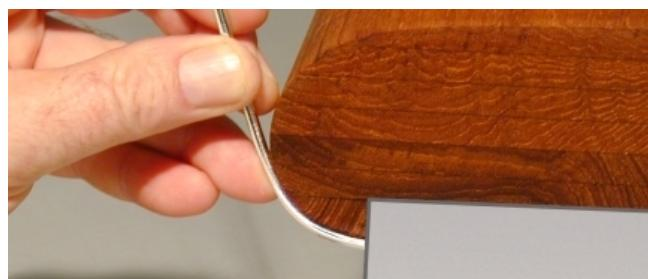
**Step 3—** Carefully bend the metal rod or strip to accurately follow the contour of the cap rail.
