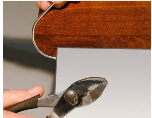
**Step 4—** Continue following contour using pliers as aid in bending rod to assure snug fit.
